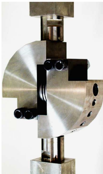
Fig. 6. Arcan type device.
